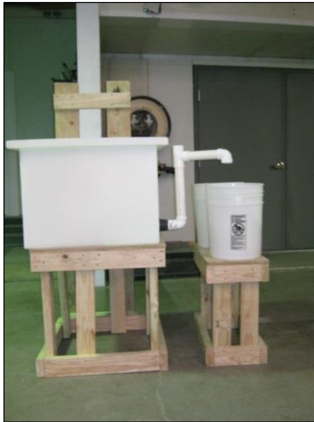
Figure A9. An image of an individual SAGB and effluent catchment system.
