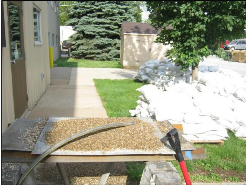
Figure A11. An image of the setup used to wash the pea gravel.
