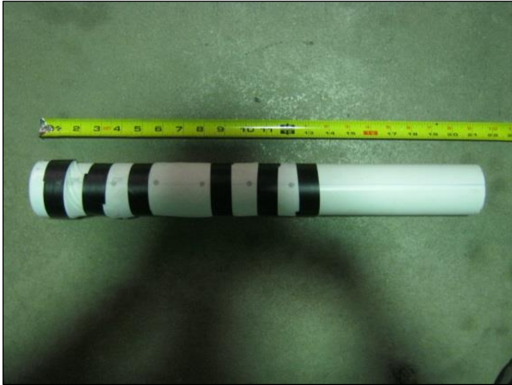
Figure A12. An image of a sample port prior to putting it into the SAGB.
